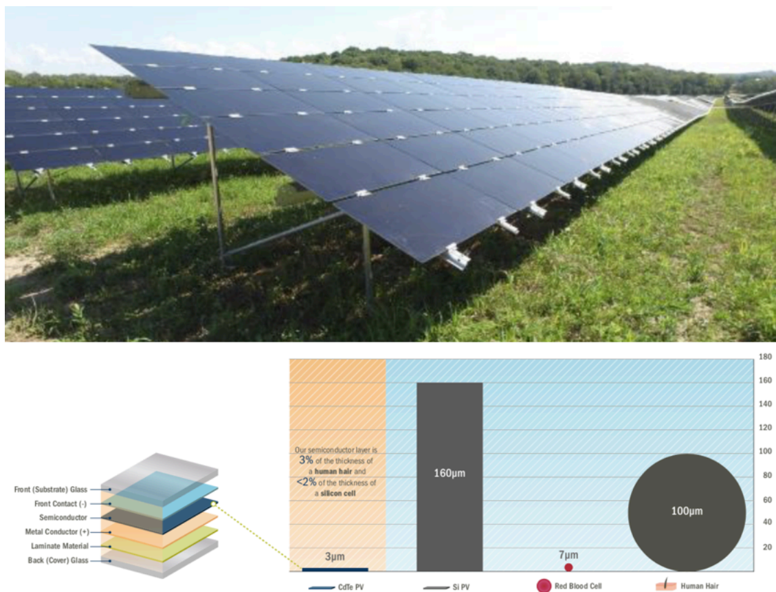
Figure 2: A CdTe photovoltaic system (top), and a schematic cross-section of a CdTe photovoltaic module (bottom). For comparison, the central CdTe layer is thinner than the thickness of the corresponding semiconductor layer in a silicon photovoltaic device, or the diameter of a red blood cell, or the thickness of human hair. Image source: First Solar, Inc.
